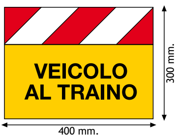
Cod. 90131 Pannello per veicoli al traino 400x300 - 1 mm. Panel for towed vehicles 400x300 - 1 mm.
